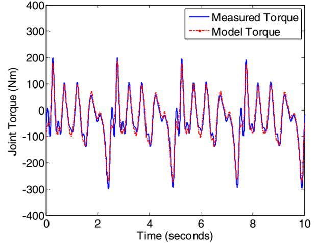
Fig. 5 Motor Torque for Joint 2
