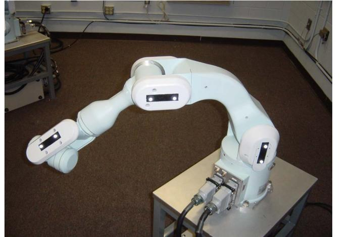
Fig. 2 Motion Capture Markers on PA10-6CE.
