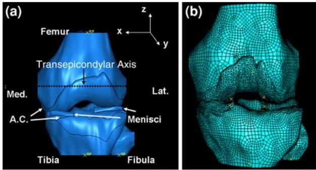
**FIGURE 2.** (a) Three-dimensional geometry of the left knee, which includes femur, tibia, fibula, articular cartilage and lateral and medial menisci with the dotted line representing the transepicondylar axis and the location where the loading was applied. (b) A typical mesh of the knee geometry.
