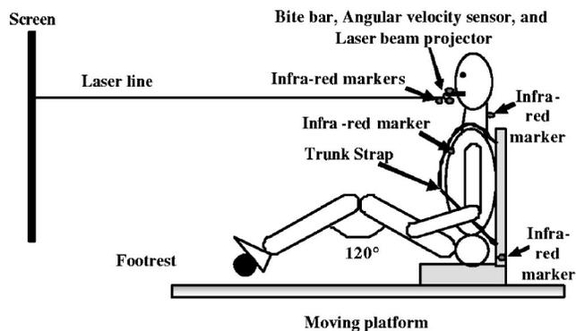
FIG. 1. An illustration of the position of the subject seated on the linear sled, the location of the infrared markers and the angular velocity sensor, and the direction of the laser beam projected on to the screen in front of the subject.
