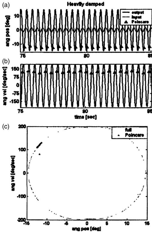
FIG. 4. Output of the model simulation for a heavily damped system with a driving frequency of 2.25 Hz. Plots are the same as in Fig. 3. Input parameters were:  $T=0.8$  N m,  $m=4.5$  kg,  $k=10$  N m/rad,  $b=0.2$  N ms/rad,  $\theta_{th}=1^\circ$ ,  $\dot{\theta}_{th}=0^\circ/s$ . 10 s period of simulations are presented in (a) and (b).
