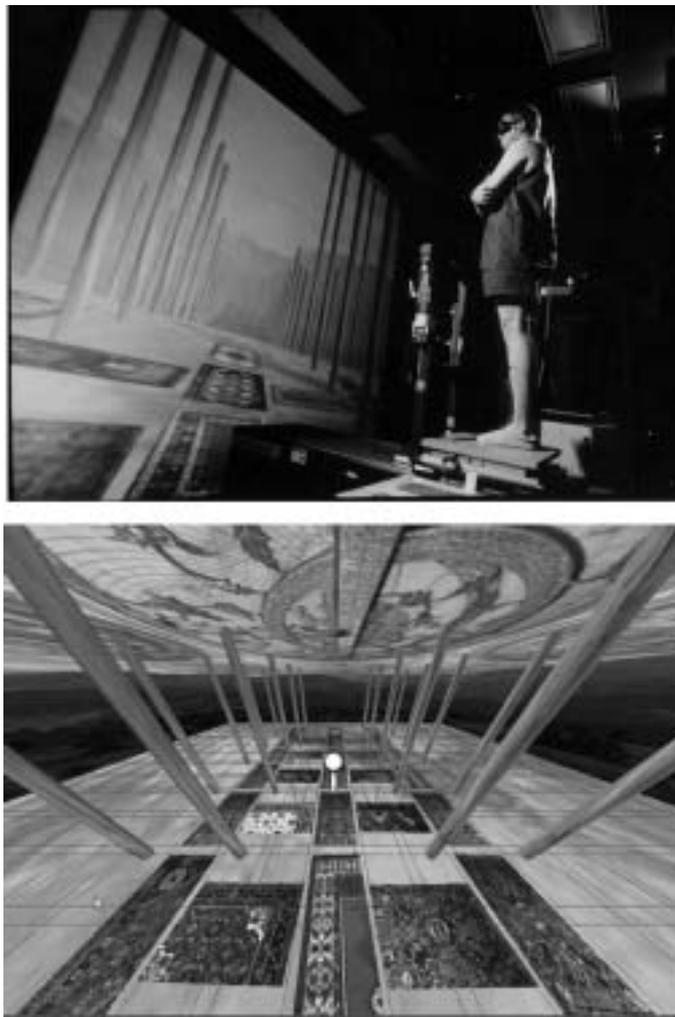
Fig. 1. Top figure shows the dynamic image presented to a subject standing on the translating sled. Subject is wearing stereographic glasses (Crystal Eyes, Qualix Direct, CA) in order to perceive the stereo image. The bottom figure is a birds-eye view of the entire image. The white circle in the center illustrates where the subject is positioned in the image. Only the portion of the image that is in front of the subject can be seen.
